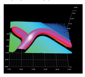
Adhesive or sealant webs applied with dispensers must meet the highest quality requirements to ensure the function of the component. NeuroCheck offers suitable sensors to record and evaluate dispensing beads in great detail. In this application, the webs are examined and measured with regard to the application thickness, height and position in relation to a reference position. The test takes place directly after the dispensing process on the component surface.
