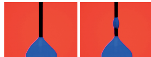
Result OK Result NOK because of remnants of adhesive on the needle shaft
